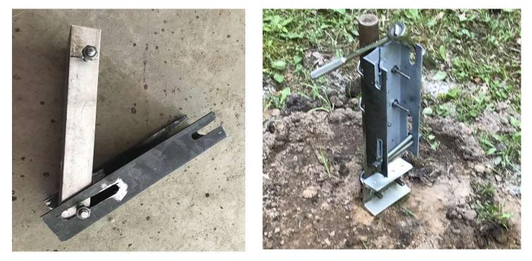
The aluminum channel at the right side of the picture was drilled and tapped for 1/4-20 bolts and would function as the radial attachment point. Using two long lag bolts, I measured and cut the required radials
