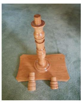
Overlooking the planned design, a unique item might be the pedestal post itself comprised of White Oak vintage lumber cut into sections and glued together to form an assembly that could be turned on a wood lathe.
